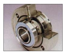
The GPEC is a cartridge type seal which has a built in ball bearing system. This provides excellent centering of the seal, since the bearing is very close to the friction surfaces.
