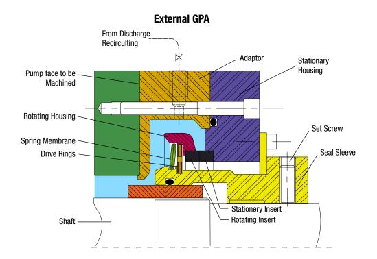
GPA® cartridge type, this specific design can be mounted outside of the pump body, in this particular case, operating at 200°F / 95°C, 1400 rpm, Suction pressure 25 PSI / 1.8 bar, discharge pressure 90 PSI / 6 bar. The seals replace the packing rings without modifications to the pump.
